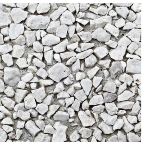
77 Washed concrete White crushed stone 4/8mm SC
